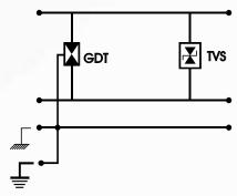
GDT: 3-electrode gas tube
