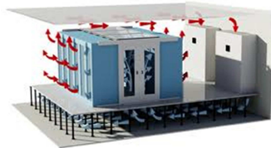
FIGURE 2: COLD AISLE CONTAINMENT ON A RAISE FLOOR
